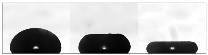
Fig. 1: Images of the surfactant drop with IP film formation during compression
